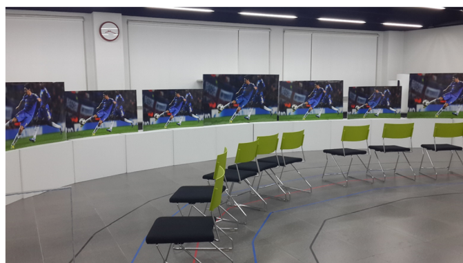
FIGURE 4 — Survey setup: nine displays and nine chairs placed initially on 2.5 m distance from the respective display.
